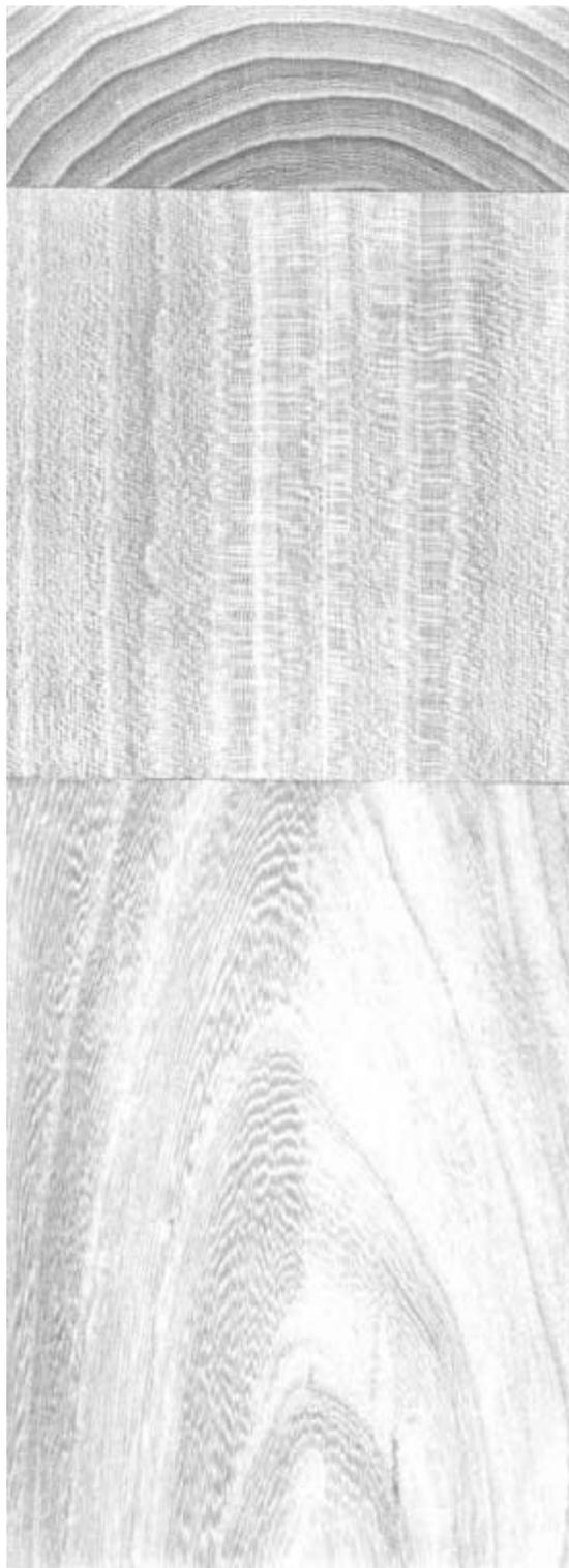
Figure 5.—Wood of American elm: top—transverse view; middle—radial view; and bottom—tangential view (plainsawed).
